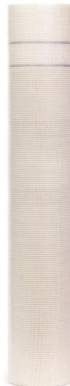
**Application:** Reinforcing glass fibre mesh for external thermal insulation systems (ETICS). The fiberglass mesh must be embedded with 10 cm overlapping, moving continually from up to down and from inside to outside in the base coat applied on the whole surface by 10 mm notched trowel, then smoothing it so that the reinforcing mesh positioned in the middle (by EPS) or in the outer third (by MW) of the base coat layer and covered completely.
